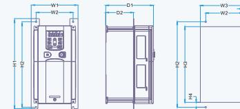
18.5-30kW Flange mounting Installation diagram
