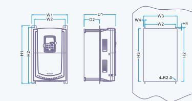
18-55kW Flange mounting installation diagram
