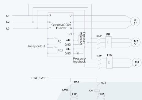
In the diagram above, M2 and M3 are auxiliary motors which are controlled by R01 and R02. PID constant-pressure automatic control system is formed by the inverter through pressure feedback. The pressure reference can apply analog or keypad input. 485 remote communications is also supported.
