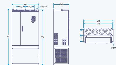
350-500kW Floor mounting Installation diagram
